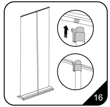
16. The plastic holder at the top of pole slips into the rear slot of the banner beam. A marker on the beam indicates the beam's centre where the pole should be inserted.
